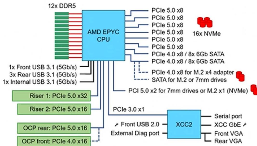
Figure 4. SR635 V3 Server Interconnect Diagram, showing major components and their connections.
