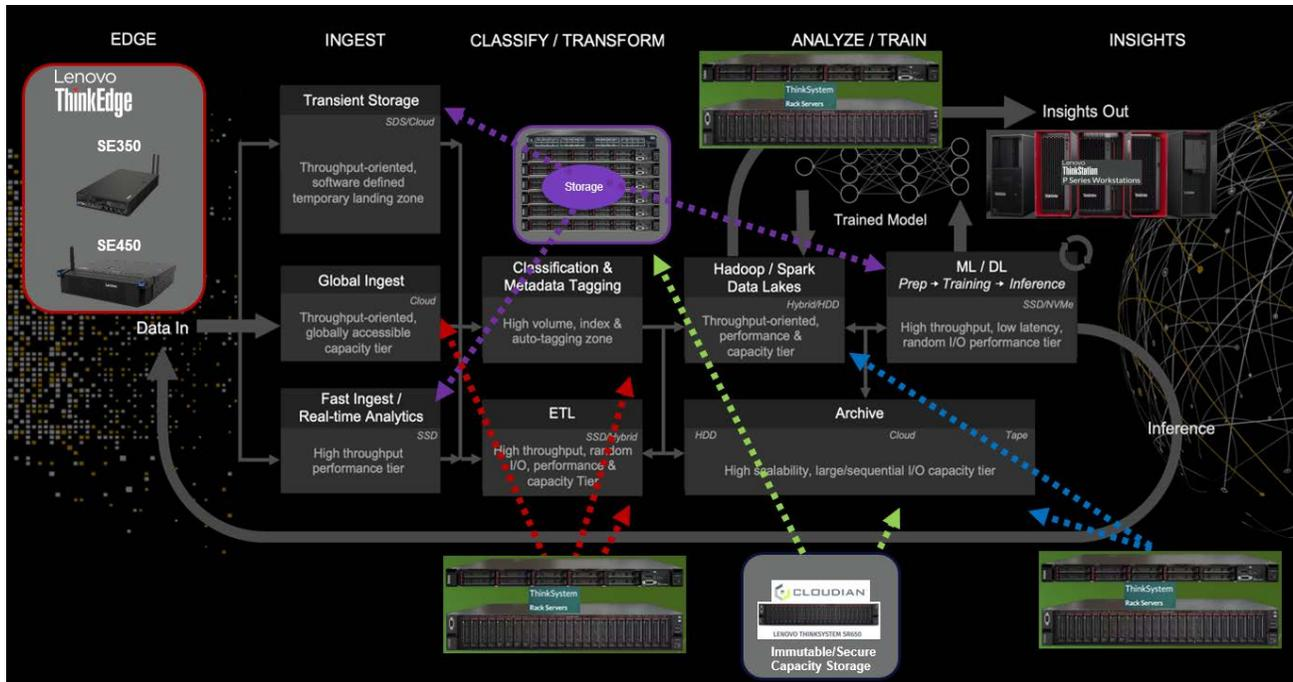
Figure 6. Analytics data pipelines enabled by Lenovo Infrastructure Solutions and leading software partners. The [Lenovo AI-Ready](#) portfolio consists of ThinkSystem servers, ThinkEdge devices, and ThinkStations. These play a role in an overall AI strategy. Below provides a description of each machine category and the most common AI personas that would use.
