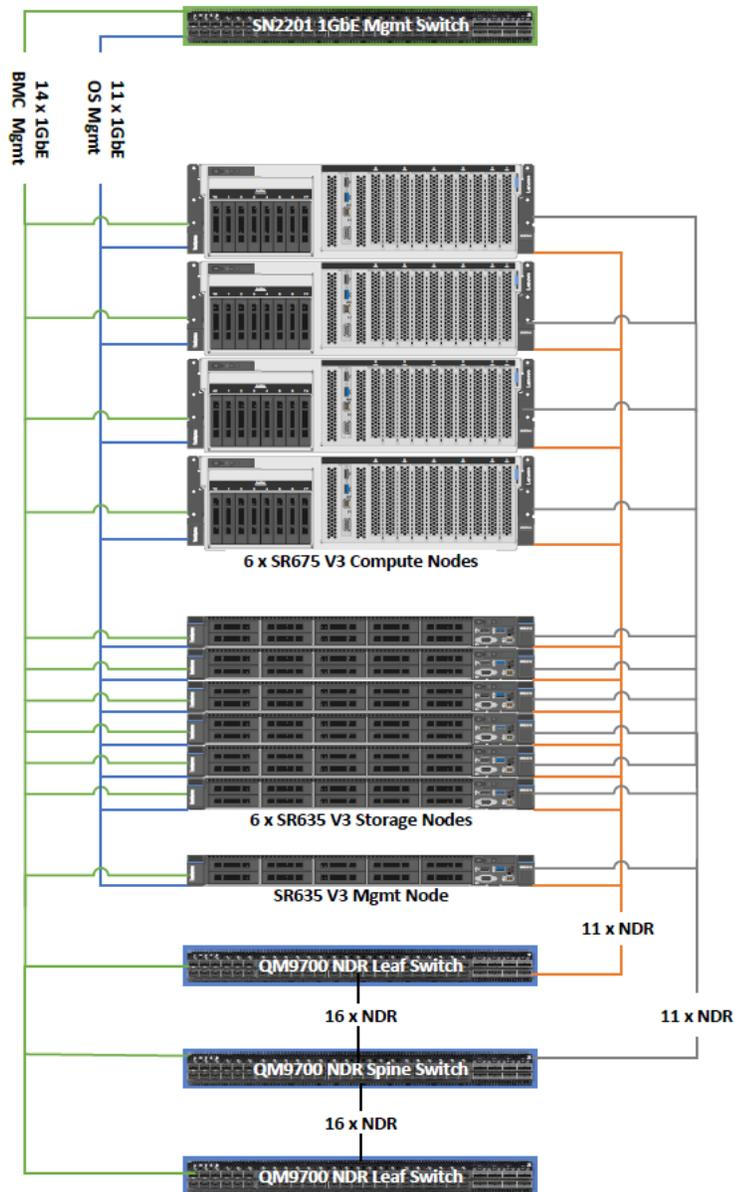
Figure 2. Rack and stack view of the reference architecture
