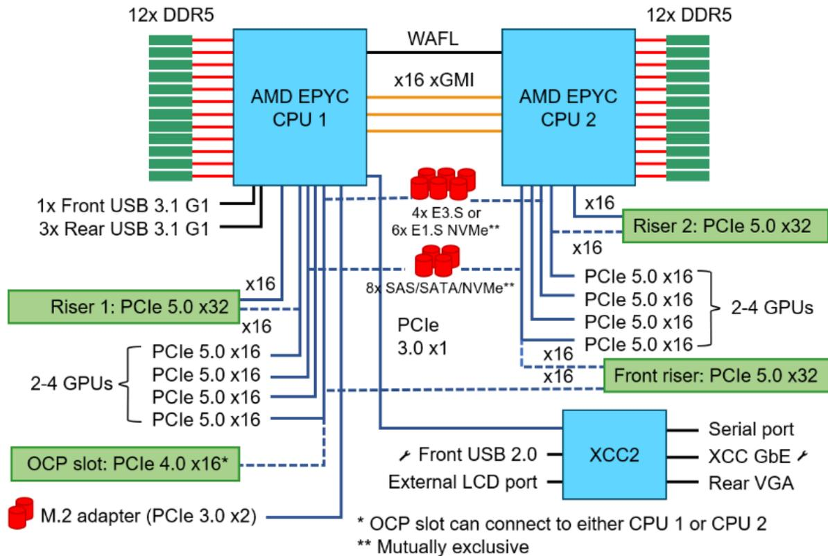
Figure 5. SR675 V3 Server Interconnect Diagram, showing major components and their connections.
